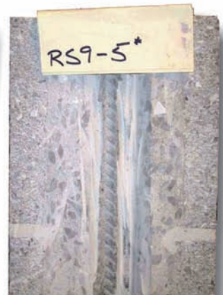
Cross section of blockwall cell using Oztec Rebar Shaker®
